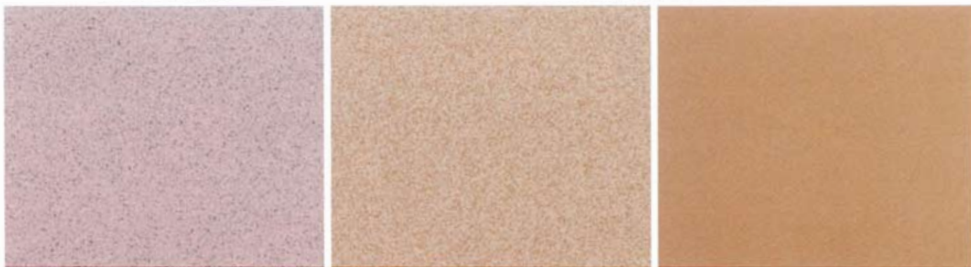
Figure 1. A variation in the number of differently coloured spray powders that comprise porcelain tiles, and their size, can be seen with small magnification of the surface.
